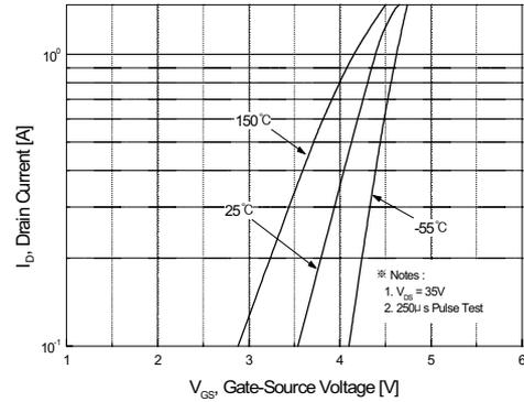
Figure 2. Transfer Characteristics
