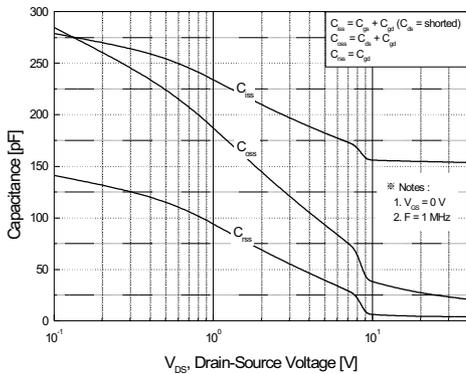
Figure 5. Capacitance Characteristics
